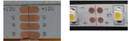
The best results are achieved with the 3M tape on the LED's, if they are applied to a clean surface. Clean all surfaces, removing any dust or oil from your plane. You can run jumpers from a set of pads in the middle of a strip to a new strip of LED's.
