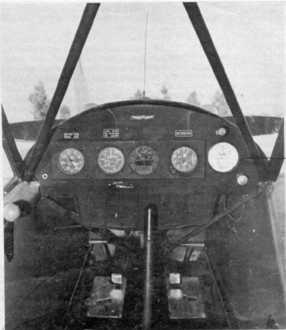
For maximum points in Stand-off Scale, this easy-to-reproduce instrument panel can be installed. This is, of course, the interior of the full-scale L-4.
